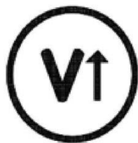
Over voltage Protection
